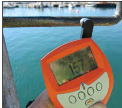
Zinc chlorides salts almost non-existent on round bar climbing hoops, coating thickness - 157µm.
