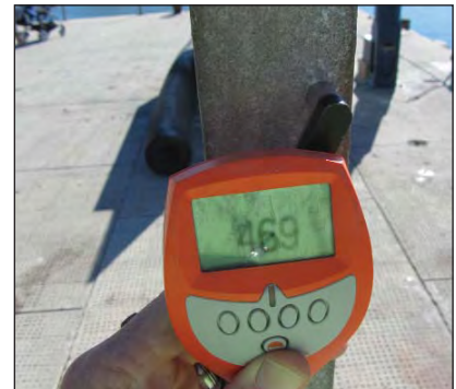
Zinc chloride layer including the hot dip galvanized coating thickness of 469µm.
