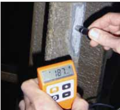
The hot dip galvanized coating thickness on station steelwork proved to be in good condition.
