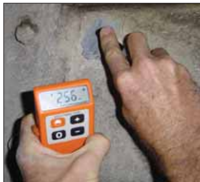
The coating thickness on shaft buntuns at four different levels were inspected but as they were similar in residual coating thickness, only two have been reported. The calcerous growth in most instances was removed prior to measuring the residual coating thickness.
