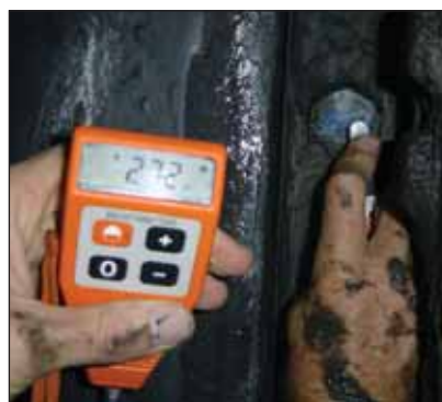
Coating thickness indicated on various parts of the shaft guides, proved that the original predicted service life of 25 years would be achieved.
