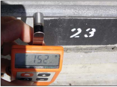
Coating thickness readings on the round bar of the seat (152 \mu m) (left), on the side support (117 \mu m) (middle) and on the seat support (114 \mu m) (right).
