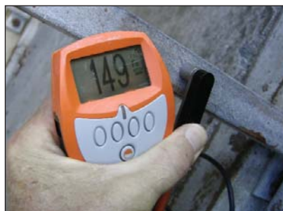
Coating thickness readings on seat side support (above left - 149 \mu m and right - 143 \mu m).
