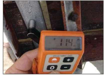
Coating thickness readings on the round bar of the seat (152 \mu m) (left), on the side support (117 \mu m) (middle) and on the seat support (114 \mu m) (right).
