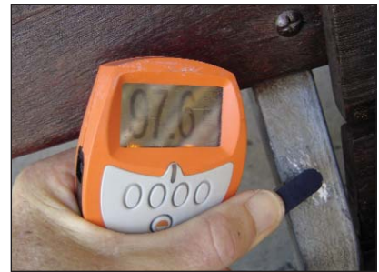
Coating thickness readings of seat side bracket (above left - 92.1 \mu m and right - 97.6 \mu m).
