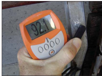
Coating thickness readings of seat side bracket (above left - 92.1 \mu m and right - 97.6 \mu m).
