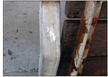
Removal of contaminants prior to taking coating thickness readings on seat side bracket.
