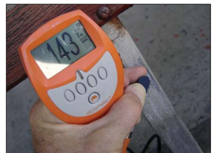
Coating thickness readings on seat side support (above left - 149 \mu m and right - 143 \mu m).
