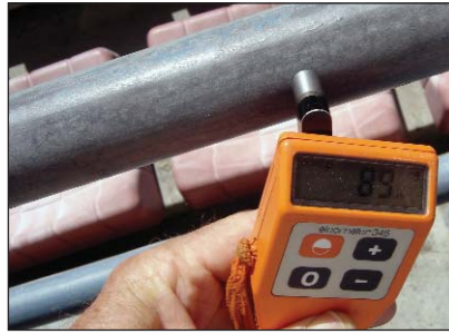
Coating thickness readings on the handrails (above left - 96.2 \mu m and right - 89 \mu m).
