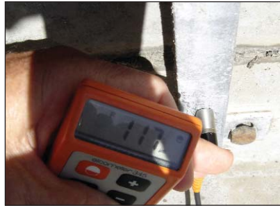
Coating thickness readings on the round bar of the seat (152 \mu m) (left), on the side support (117 \mu m) (middle) and on the seat support (114 \mu m) (right).
