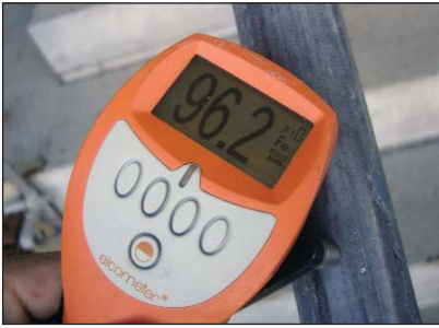
Coating thickness readings on the handrails (above left - 96.2 \mu m and right - 89 \mu m).
