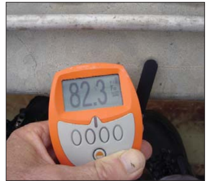
Photos above show coating thickness on the side rails (89.6 and 82.3µm) and again on the cross rung (82.3µm). Coating thicknesses are still well above that required by the standard.
