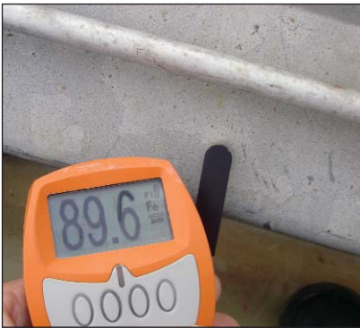
Photos above show coating thickness on the side rails (89.6 and 82.3µm) and again on the cross rung (82.3µm). Coating thicknesses are still well above that required by the standard.
