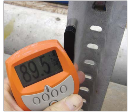
Photo left shows the A&S Cable ladder in the foreground and a more modern edge mounted cable ladder in the background. Centre shows a close up of the A&S Cable ladder and right, residual coating thickness on the cross rung (89.5µm).
