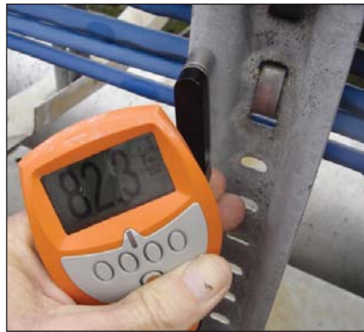
Photos above show coating thickness on the side rails (89.6 and 82.3µm) and again on the cross rung (82.3µm). Coating thicknesses are still well above that required by the standard.
