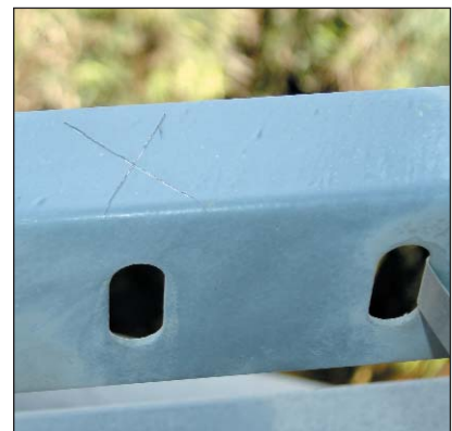
Exposed powder coating subjected to a cross cut adhesion test.
