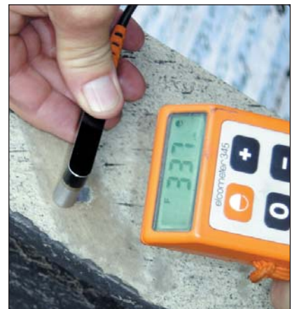
Total duplex coating thickness.
