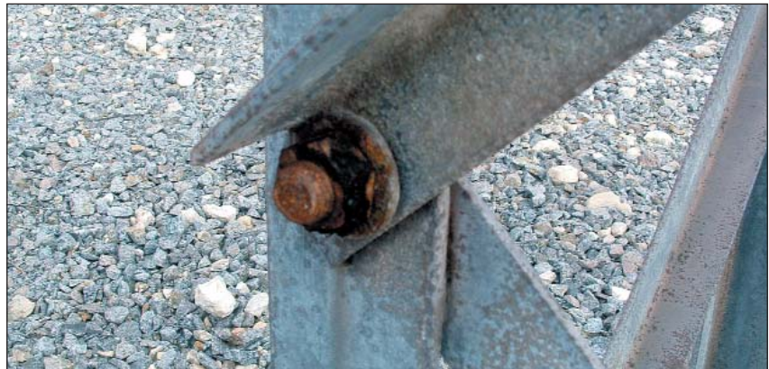
Despite the apparent "rust" contamination of the galvanized surface, once removed the galvanized coating measured 126µm.
