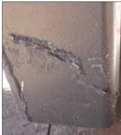
Photos above show unacceptable coating roughness and a zinc run at the weld area, which should ideally have been removed prior to painting.
