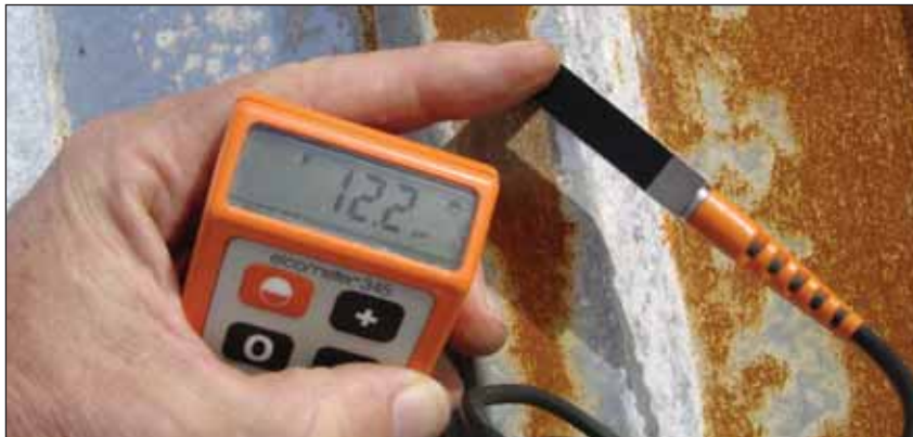
Coating thickness is just below the minimum prescribed in SANS 3575, which for Z275 is 13.5µm.
