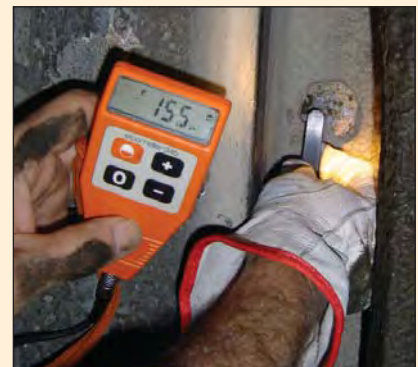
Coating thickness indicated on various parts of the shaft guides, proved that the original predicted service life of 25 years would be achieved.
