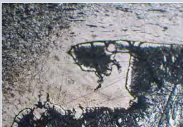
Figure 5: Zinc filling at the welded joint (125x).
