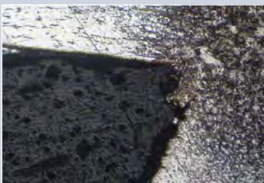
Figure 7: Burn back of the zinc layer at the welded joint (125x).
