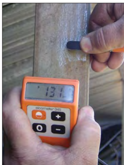
Coating thickness readings taken on all the horizontal and vertical overland conveyor steelwork were still in excess of that required by the specification.
