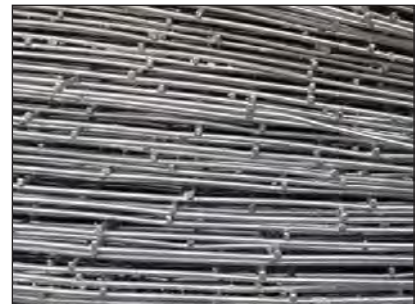
Photo above left shows excessive amount of zinc most probably situated at the lower end of the mesh as they hung on the flight bar, whereas the photo on the right shows the relatively clean and free from excessive zinc which more than likely was at the upper end of the mesh as they hung on the flight bars, when exiting the bath of molten zinc.
