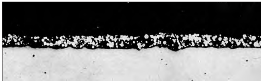
Typical section through a zinc rich paint layer.
