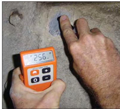
The coating thickness on shaft buntons at four different levels were inspected but as they were similar in residual coating thickness, only two have been reported. The calcerous growth in most instances was removed prior to measuring the residual coating thickness.
