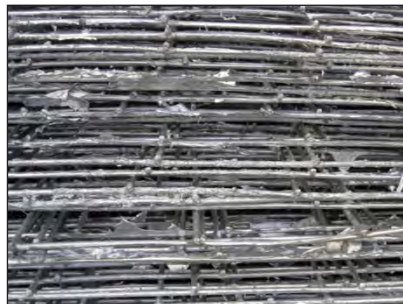
Photo above left shows excessive amount of zinc most probably situated at the lower end of the mesh as they hung on the flight bar, whereas the photo on the right shows the relatively clean and free from excessive zinc which more than likely was at the upper end of the mesh as they hung on the flight bars, when exiting the bath of molten zinc.
