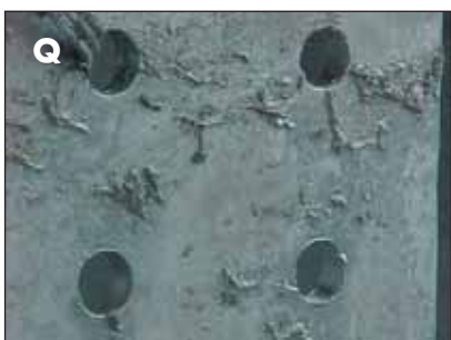
Ash deposits on mating surfaces.
