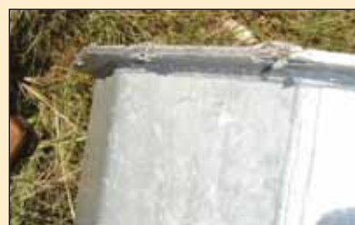
The above photos 25 - 32 (clockwise from top left) indicate the extent of mechanical damage (where some residual iron/ zinc alloy layers remain intact) to the coating and in some instances non-damage at scuffmarks.
