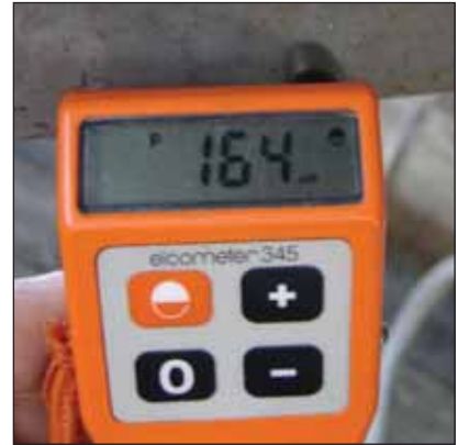
Coating thickness on the tube for the treatments/artificial insemination stall after 6 years of exposure.
