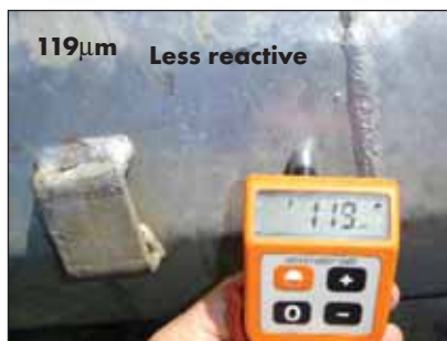
Photos 23 (left) and 24 (right) indicate the difference in coating thickness readings for both the less reactive and more reactive steels, respectively.
