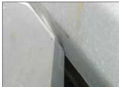
Photos 16, 17 18 and 19 (clockwise from top left) show how inappropriate stacking on site, particularly when weld on gusset plates and sharp corners clash, can cause coating damage.
