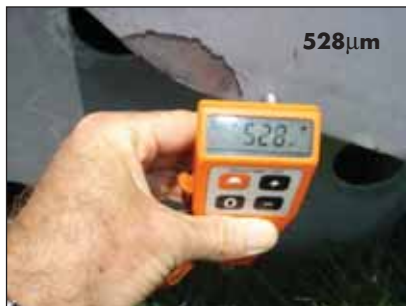
Photo 4. Coating thickness reading (528 \mu m) on the base plate steel adjacent to mechanical damage.
