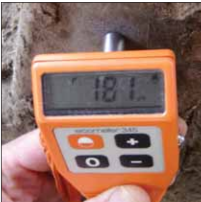
Cattle dung removed from the base of the cattle separation barrier post and coating thickness measured.
