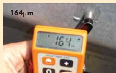
The coating at some of the scuffmarks (photos 33 & 34) was not necessarily damaged sufficiently to warrant repair.
