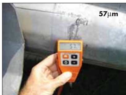
Photo 3. Coating thickness reading measuring the residual iron/zinc alloy layer (57 \mu m) at a mechanically damaged area.
