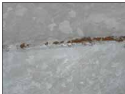
Photos 9, 10 and 11 (left to right). Mechanically damaged coatings due to inappropriate transportation, handling and stacking.
