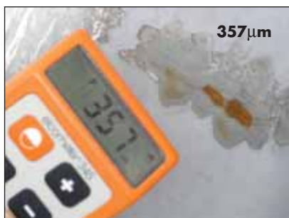
Photo 2. Coating thickness reading on the surrounding coating (357 \mu m) adjacent to mechanical damage.
