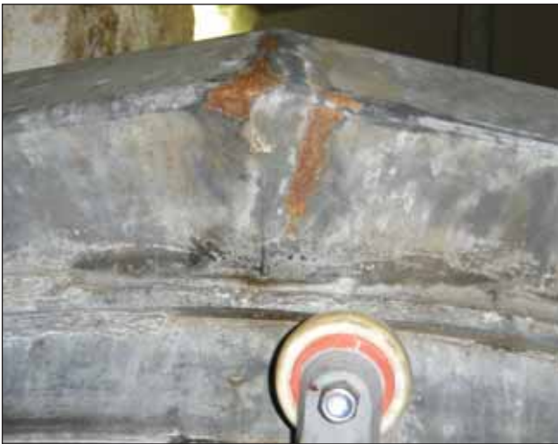
Alterations and coating repairs must be kept to a minimum particularly in this type of application. Here the coating repair material that was used has failed and must be redone with a more suitable material.
