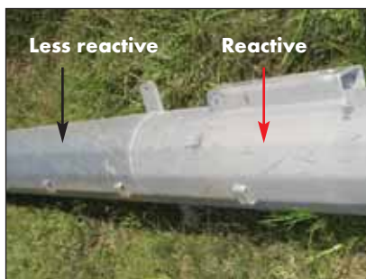
Photo 22 shows the reactive steel on the right of the mast, with the less reactive steel on the left.
