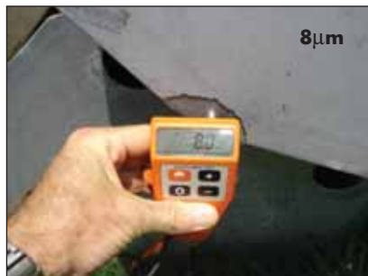
Photo 5. Coating thickness reading measuring the residual iron/zinc alloy layer (8 \mu m) at the mechanically damaged area on the base plate.
