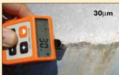
The above photos 25 - 32 (clockwise from top left) indicate the extent of mechanical damage (where some residual iron/ zinc alloy layers remain intact) to the coating and in some instances non-damage at scuffmarks.
