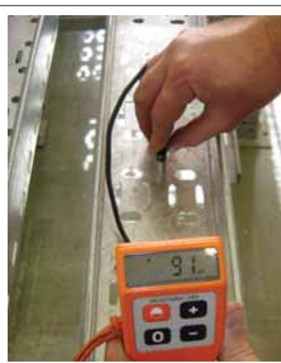
Although both cable trays are hot dip galvanized the tray on the left has been manufactured from continuously hot dip galvanized sheeting, coating class Z275 (coating thickness 16.9µm) and the tray on the right hot dip galvanized to SANS 121 (coating thickness 91µm).
