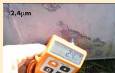
Photos 23 (left) and 24 (right) indicate the difference in coating thickness readings for both the less reactive and more reactive steels, respectively.
