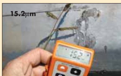
Photos 23 (left) and 24 (right) indicate the difference in coating thickness readings for both the less reactive and more reactive steels, respectively.
