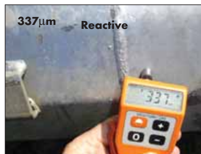
Photos 23 (left) and 24 (right) indicate the difference in coating thickness readings for both the less reactive and more reactive steels, respectively.
