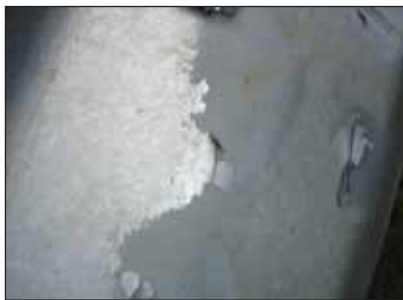
Photos 12 (left) and 13 (right). Abrading of the hot dip galvanized surface prior to zinc metal spraying is of major importance to ensure adhesion of the zinc metal sprayed coating. Furthermore, it is important that excess zinc metal spraying, that adheres to non-prepared surfaces be removed by stainless steel wire brushes, prior to delivery by the galvanizer.
