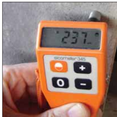
Hot dip galvanized coating thickness on the structural steel in the feeding shed.
