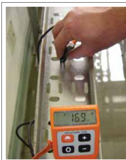
Although both cable trays are hot dip galvanized the tray on the left has been manufactured from continuously hot dip galvanized sheeting, coating class Z275 (coating thickness 16.9µm) and the tray on the right hot dip galvanized to SANS 121 (coating thickness 91µm).
