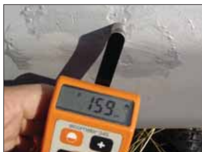
Photos 42 (left) and 43 (right) The coating thickness for most of the repairs was in accordance with the specification.
