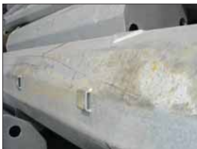
Photos 14 (left) and 15 (right) – scuff marks on the sides of some of the masts.
