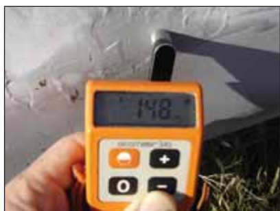
Photos 42 (left) and 43 (right) The coating thickness for most of the repairs was in accordance with the specification.
