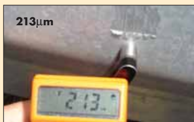
The coating at some of the scuffmarks (photos 33 & 34) was not necessarily damaged sufficiently to warrant repair.
