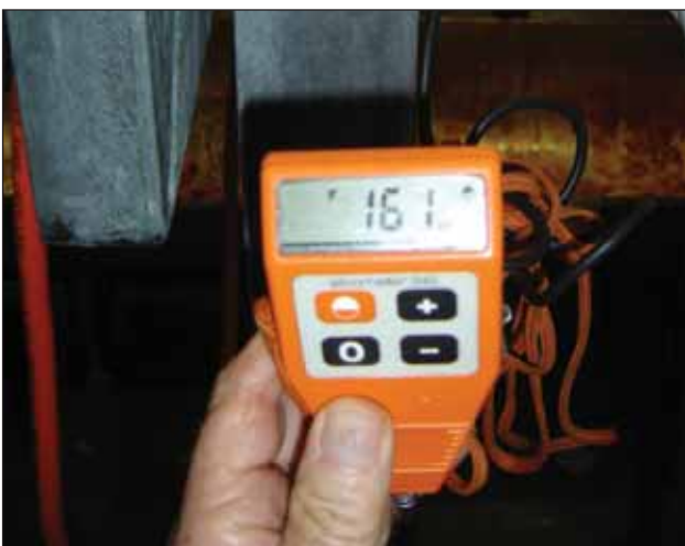
Coating thickness on this structural steel is still far in excess of the minimum required by the specification (70µm), in spite of its exposure to this atmosphere for more than 6 years and continual wash down of the structure with the cleaning chemical.
