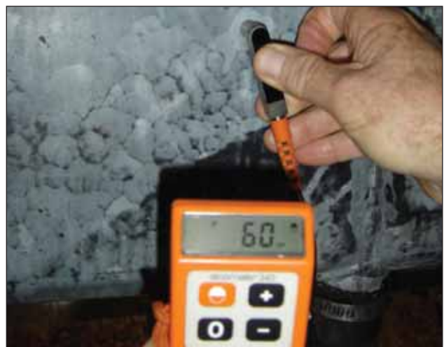
The hot dip galvanized coating on the 2mm thick edge plate of this walk way has been reduced by about 10µm over the 6 years of exposure (about 1.5µm per year). This is in spite of the aggressive wash down method that is used to produce clean surfaces, required by authorities.
