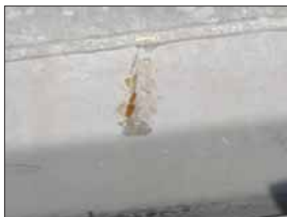
Photos 9, 10 and 11 (left to right). Mechanically damaged coatings due to inappropriate transportation, handling and stacking.
