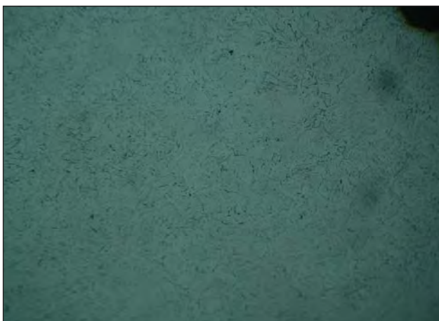
Figure 7: Cross section through the weld and heat affected zone (125X). Note the coarse acicular grain structure.
