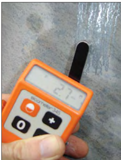
Minimum coating thickness, 2.7mils (68µm) on panel.
