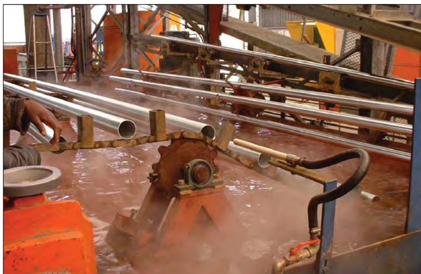
Hot dip galvanized pipes being conveyed to be quenched and passivated in order to prevent white rust also referred to as wet storage stain.
