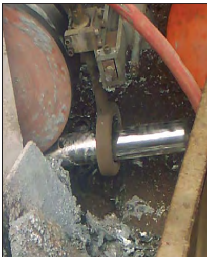
A hot dip galvanized pipe passing through the air blowing ring and being wiped.
