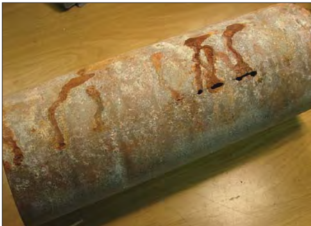
Figure 1: Section of underground pipe as received. Note the white (zinc) corrosion product and red rust emanating from the longitudinal perforations associated with the weld seam.
