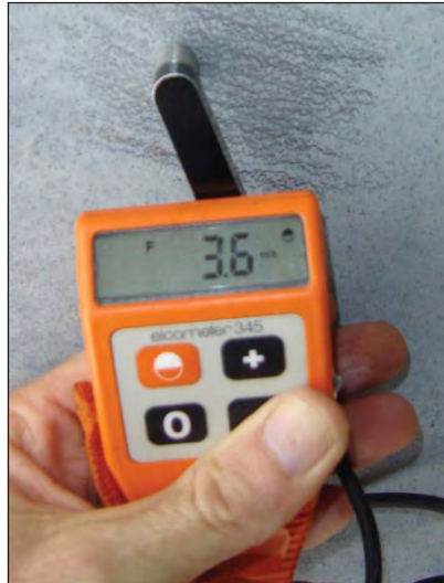
Maximum coating thickness, 3.6mils (91µm) on panel.
