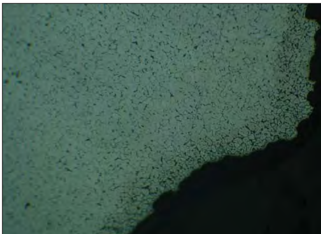
Figure 5: Cross section through the corroded region (125X). Note the clean ferrite structure.
