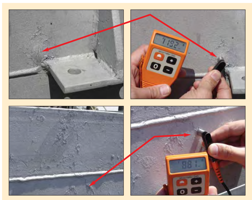
Figure 1: Lumps and runs leading to excessive coating thickness.
