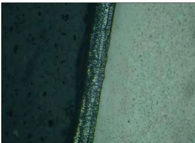
Figure 6: Cross section through the external surface galvanized zinc skin (125X). Note the various zinc-iron alloy layers present in the coating.
