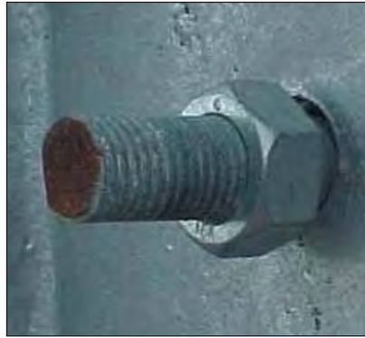
Unless repaired the cut end of a hot dip galvanized threaded rod must rely on the sacrificial protection of the surrounding zinc coating.
