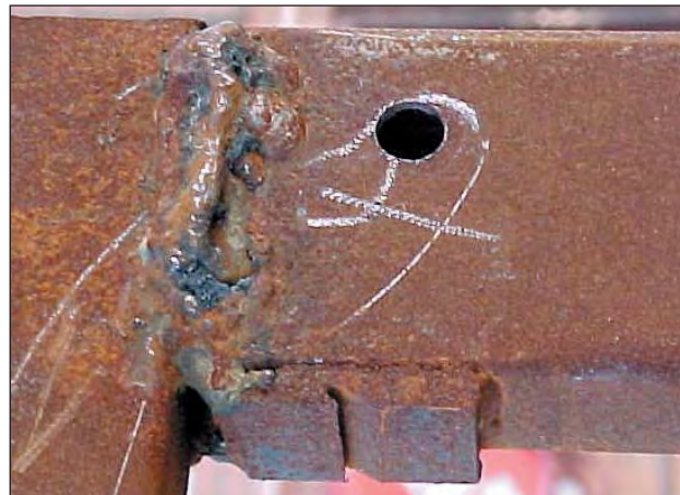
Fabrication standard and positioning of vent & fill holes has a direct impact on the quality of the hot dip galvanized coating.
