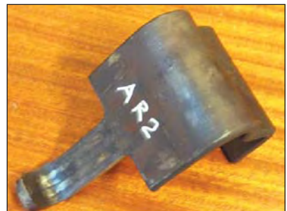
As received mild steel shoulder.
