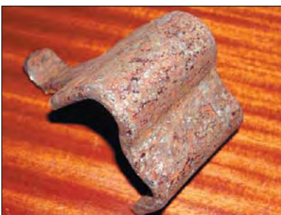
3CR12 steel shoulder after cleaning.
