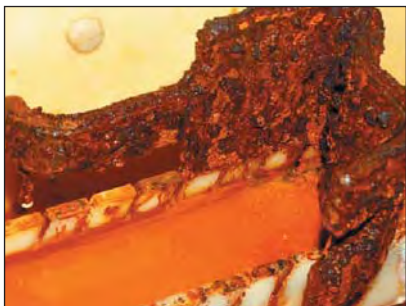
Mild steel shoulder after 1 000 hours of testing.
