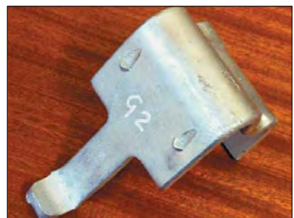
As received hot dip galvanized mild steel shoulder.
