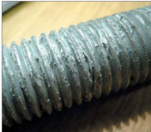
When rolling tools become worn and are not refurbished, small loosely adhering steel particles or laps are formed and after hot dip galvanizing are highlighted
