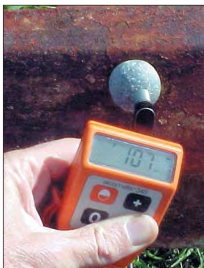
Residual coating thickness on the bolts was still about 100µm (107µm shown in photo).
