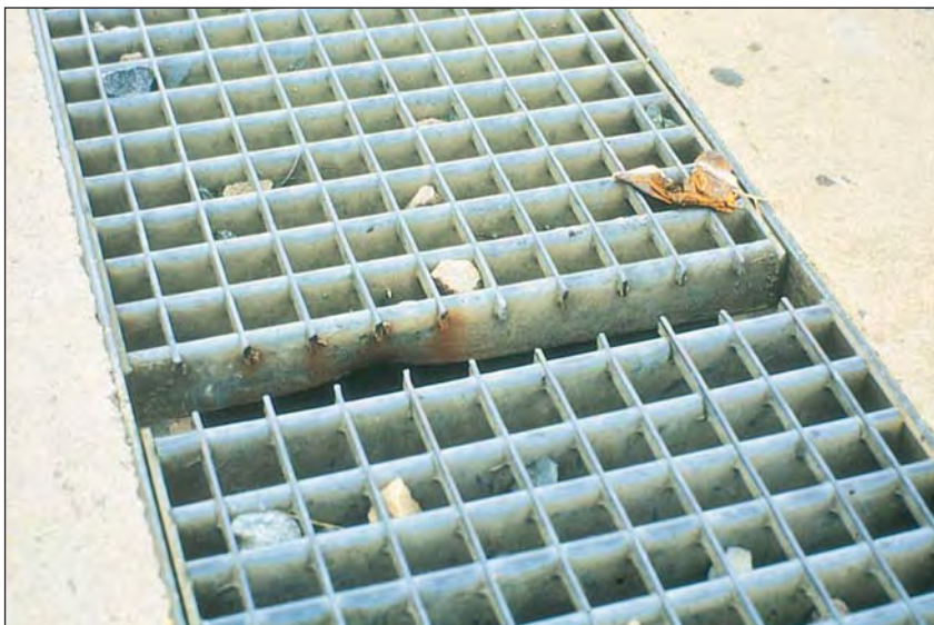
Figure 12. After 20 years of marine exposure, this site cut unrepaired hot dip galvanized steel grating still offers cathodic protection at the cut ends. The grating is now 28 years old and at the cut ends is still being protected by the surrounding coating.
