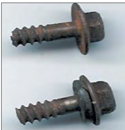
Poor fastener quality including hydrogen embrittlement can be the cause of shearing of fasteners.
