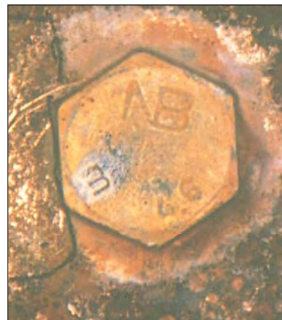
Figure 10. Hot dip galvanized bolt in contact with 3CR12 plate after 10 cycle SO 2 test. Note the cathodic protection provided by the hot dip galvanized bolt head to the surrounding steel.
