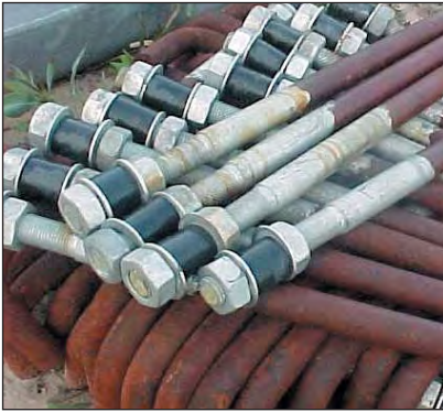
Hot dip galvanizing of only the exposed end of a holding down bolt is neither cost effective nor practical from the manufacturer and galvanizers perspective.
