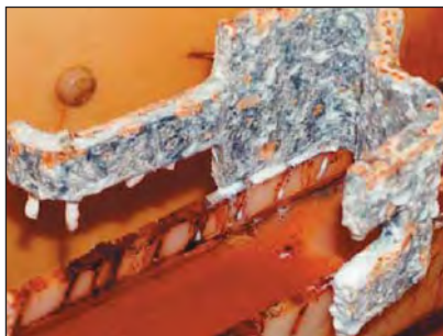
Hot dip galvanized mild steel shoulder after 1 000 hours of testing.
