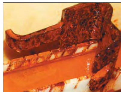
3CR12 shoulder after 1 000 hours of testing.
