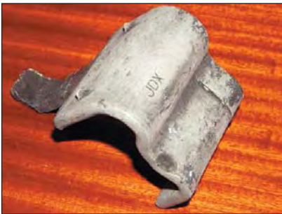
Hot dip galvanized mild steel shoulder after cleaning.
