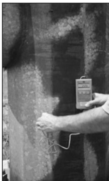
Figures 30 and 31. The galvanized coating is sometimes not uniformly grey but has a blotchy appearance with a mixture of matt, grey and shiny areas. Signs of red rust staining after several years in service is not necessarily an indication that the coating has corroded away.
