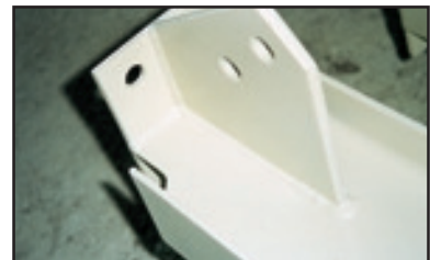
Figure 114. Sweep blasted hot dip galvanized coating followed by an appropriate paint system.
