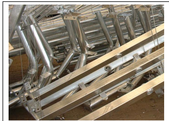
Coating thickness range between 50 to 70µm and surface finishes have a bright silvery shine. Given time (3 to 4 months exposure) all surfaces form a uniform dull grey patina of ZnCO 3 , refer to Information Sheet No. 11 “How does zinc protect?”
