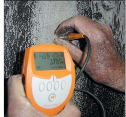
This 378µm coating reading was typical of that found on the structural steel.
