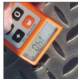
Photo 7 shows the close-up appearance of the "Vastrap Plate" and photos 8 and 9 show the coating thickness readings taken on the anti-skid ridges of the "vastrap plate" ( $116$  to  $140\mu\text{m}$ ).
