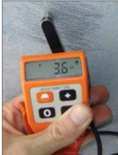
Maximum coating thickness, 3.6mils (91 \mu m) on panel.
