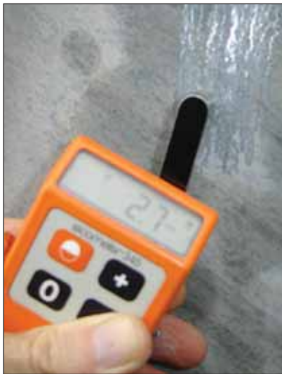
Minimum coating thickness, 2.7mils (68 \mu m) on panel.
