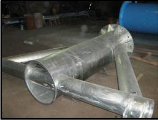
(Left and Right) Components were cleaned with grinders fixed with flexible discs.
