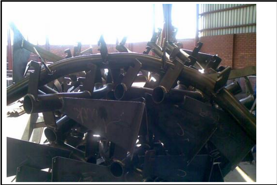
Black Steel inspected and ready for dispatch to the Galvanizers
