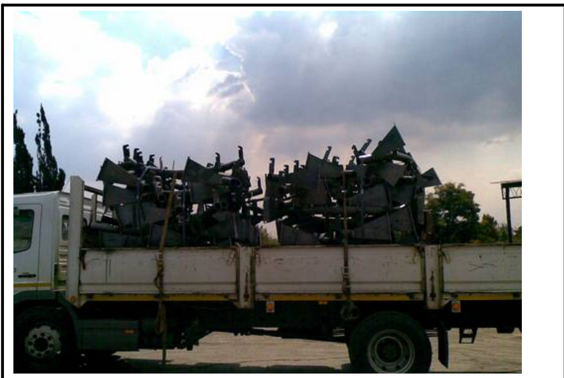
Even the black steel is strapped and loaded on smaller loads to avoid damage during transport
